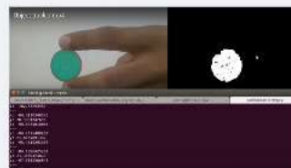
Fig. 6. Blob detection using Monocular Camera
